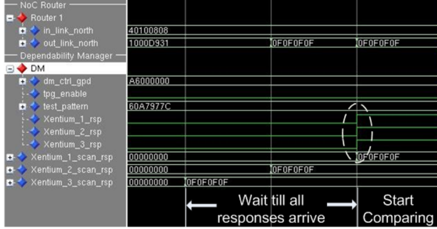
Figure 6.12: Post-synthesis simulation results of the handling of the test-responses from multiple Xentiums
